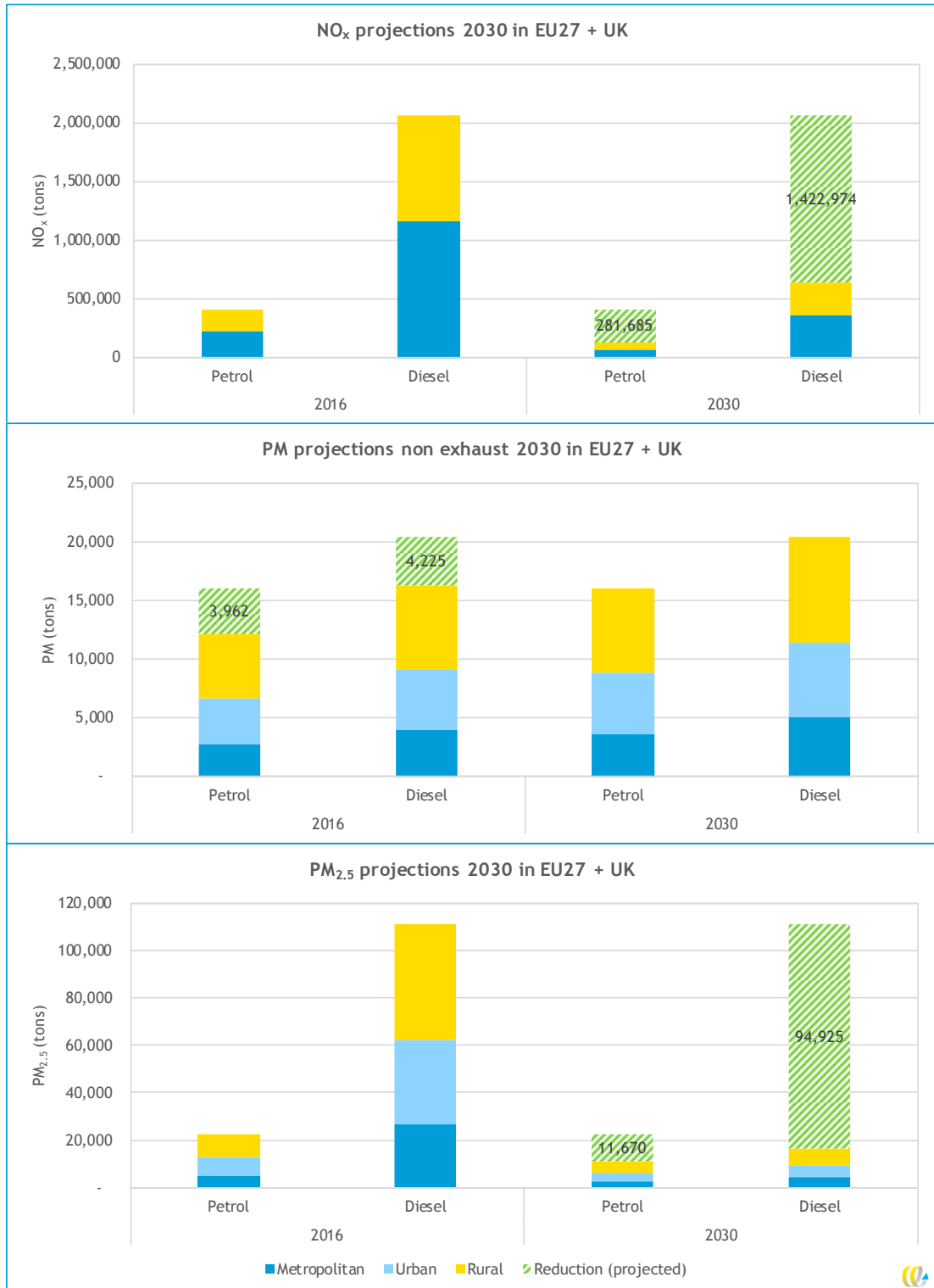
Figure 15 - NO x and PM projections in 2030 compared to 2016 based on Gains database (IIASA, 2018)
